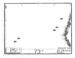
Experiment with the Wide Side transducer while operating it in a familiar area and learn how to make maximum use of the information displayed. Remember, if you are using a trolling motor mount, the information displayed is controlled by the direction the trolling motor is pointing, not necessarily the direction the boat is travelling.
